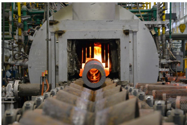
A 155mm artillery tube enters a heat treatment furnace at Watervliet Arsenal in New York.
